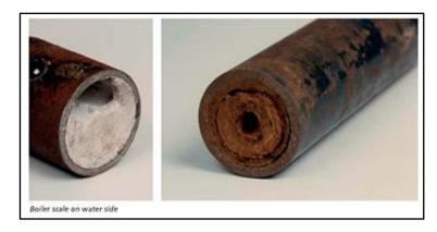
Figure 1: Scaling on pipes [2]
