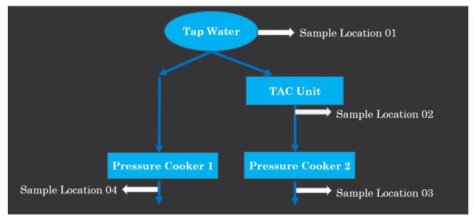
Figure 5: Experimental design set up- Flow chart
