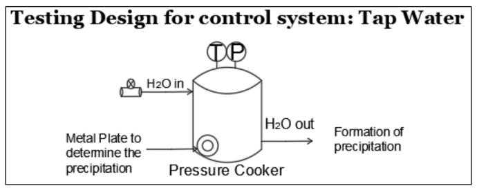
Figure 6: Experimental design control– Hard water (TAP) forms insoluble precipitates (scale) under high temperature (T) and high pressure (P)
