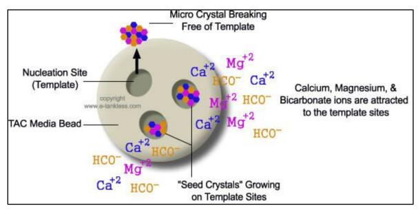
Figure 2: Example of the formation of non-reactive crystals on a nucleation site, How Template Assisted Crystallization (TAC) Filters Work [3]
